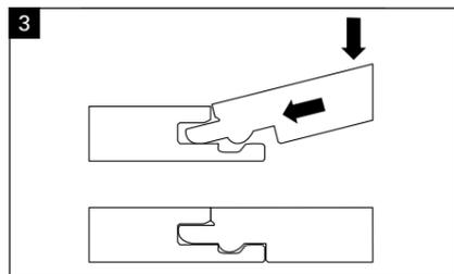
**Fig. 2 + 3:** Begin the second row on the left side by clicking the longitudinal tongue of the first board into the groove of the first row. To do so, insert the tongue into the groove at an angle of approx. 25° and lower the board. As it is lowered the board snaps into place tightly giving you a press fit.
