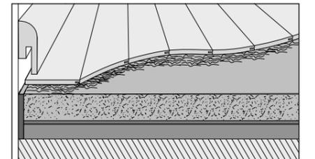
Engineered Wood Flooring, all-over adhesion
