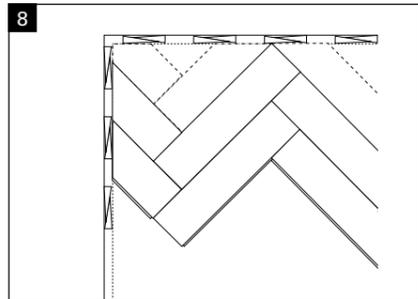
**Fig. 8:** Cut-to-size flooring pieces are used to fill the triangular-shaped spaces along the walls.
