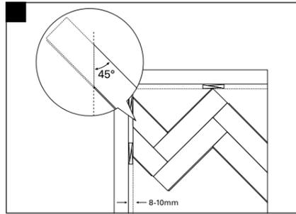
**Fig. 7:** Fit the corner planks. Saw off at a 45° angle or according to the course of the wall.
