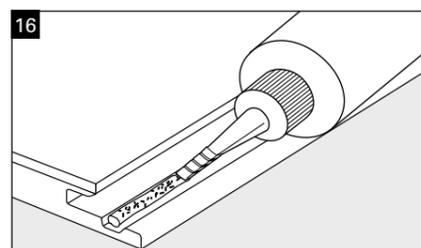
**Fig. 16:** Applying glue: If the subfloor requirements according to the country-specific standard as regards evenness (3mm/1m) or the relative humidity (35-60%) are outside the tolerances specific to the engineered wood floor, it is recommended to apply glue (see drawing).
