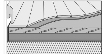
Engineered Wood Flooring on Uno-Protect / Hardwood planks
