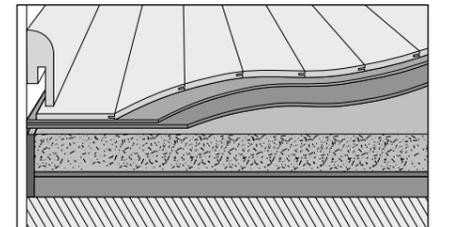
Engineered Wood Flooring on Uno-Protect / PVC / Mineral screed
