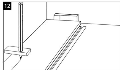
**Fig. 12:** If the wall is not straight: align the first row straight ahead and follow the contours of the wall. To do so, mark the relevant width on the plank (as shown in the diagram), and cut the plank along the mark.
