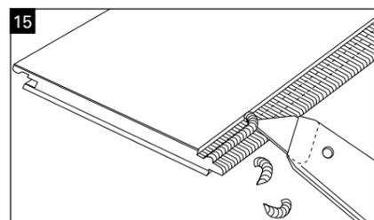
**Fig. 15:** Installation in inaccessible areas: whenever the boards cannot be swiveled in and clicked together, it is recommended to remove the catch-mechanism on the backside of the tongue and glue the boards together. Apply the glue onto the lower part of the groove and join the boards together horizontally (conventional tongue-groove principle).
