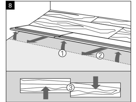
**Fig. 10:** Use a piece of residual board to help fit the last row. Remember to keep an expansion space of 10-15mm to the wall.
