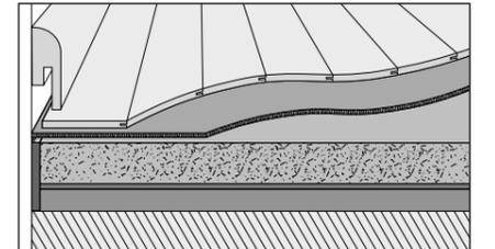
Engineered Wood Flooring on Duo-Protect / Mineral screed
