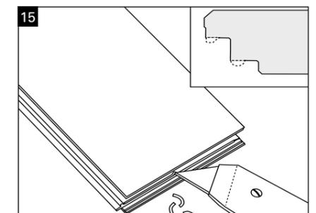
**Figure 16: Dismantling:** Should it be necessary to dismantle the floors, the glued areas must be removed first. After that the planks can be easily removed.
