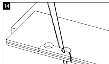
**Fig. 14:** How to fit your floor around heating pipes: the diameter of the hole in the board should be 20 mm larger than the pipe itself. Mark the spot, drill the holes and saw off at an angle of 45° as shown in the illustration. Glue in the sawn off piece. Don't forget the expansion gap here either.
