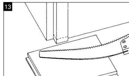
**Fig. 13:** How to shorten a door frame: place a piece of residual board (on the suitable subfloor/ underlay) against the frame and saw the frame off along the board.
