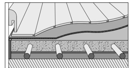
Engineered Wood Flooring on Duo-Protect / Hot water-type subfloor heating
