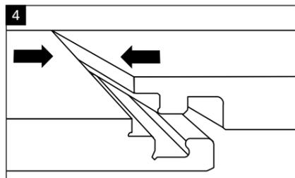
**Fig. 4:** The next board – and all the others that follow – is inserted lengthwise as described above and before lowering the short end side is positioned flush with the previous board. The solid upper wear layers need to be touching each other!
